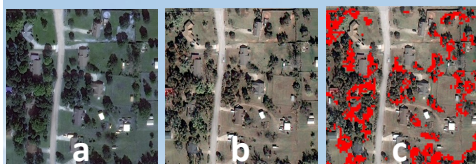
Fig. 2. High-resolution (0.5 m) Oklahoma City images (a) before storm Oct. 11th, (b) after storm Nov. 1st, and (c) detected changes.
