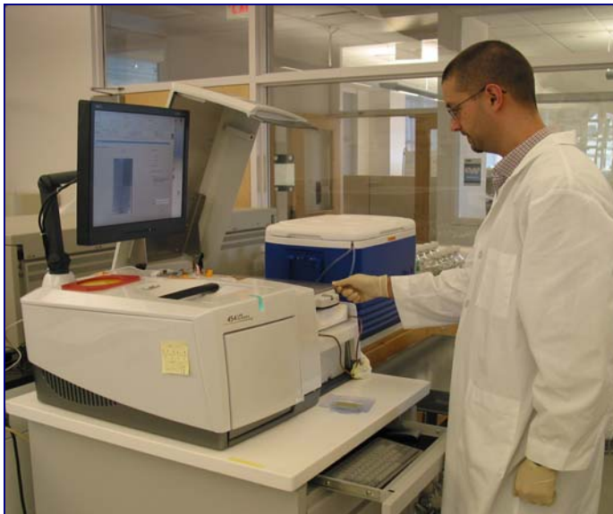
Left: Graham Wiley, in Dr. Bruce Roe's lab, loads the new 454 sequencing instrument capable of analyzing three- to four-hundred thousand templates in one day. Photo courtesy Bruce Roe.
