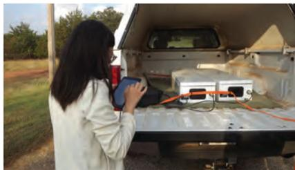
*Pictured above: Cosmic-ray neutron rover, currently in the testing stage, will be used to map soil moisture.*
