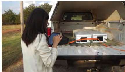
Pictured above: Cosmic-ray neutron rover, currently in the testing stage, will be used to map soil moisture. Photo credit: Yohannes Tadesse Yimam
