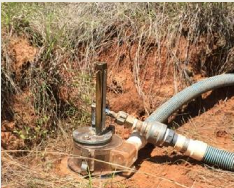
Figure 3. Controlled-burn truck used to provide water to field site (left), head tank that delivers constant pressure to JET and recycle loop to send water back to tank (middle), and JET device employed in the field with both intake and waste hose (right)
