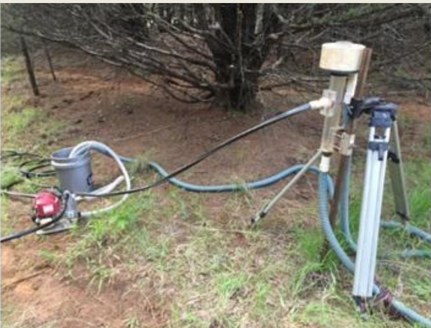
Figure 3. Controlled-burn truck used to provide water to field site (left), head tank that delivers constant pressure to JET and recycle loop to send water back to tank (middle), and JET device employed in the field with both intake and waste hose (right)
