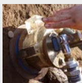
JET apparatus used to measure erodibility parameters
