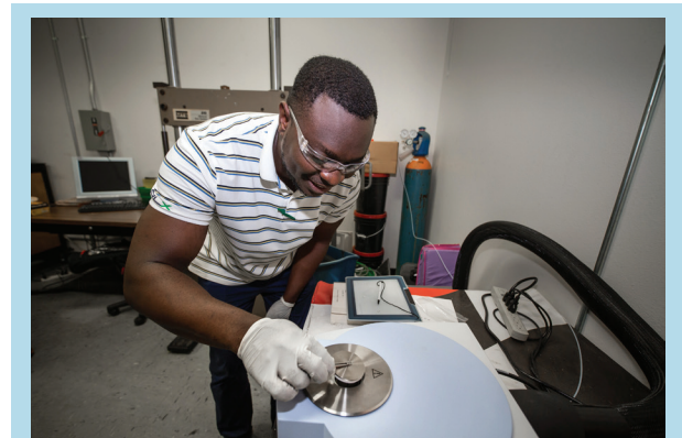
Ukeamezhim Ayaugbokor uses a high-temperature differential scanning calorimeter to analyze process conditions for advanced composite materials. Credit: Eddy Perez, LSU Strategic Communications
